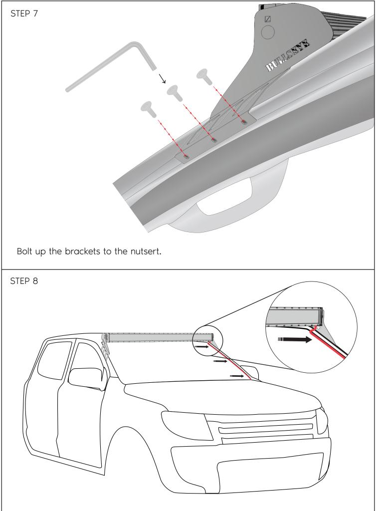
Run the wiring down the side of your windscreen, preferably on the same side as the battery. Use a few dabs of silicone or to hold it in place.
