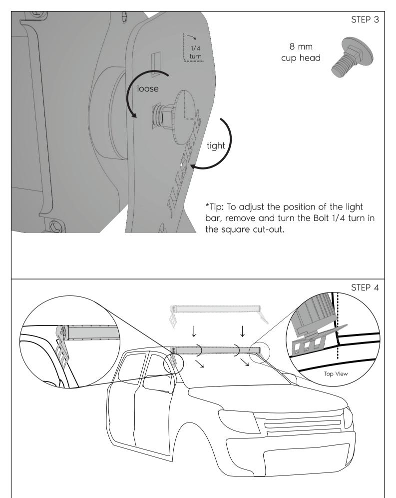
Place light bar into position on top of the windscreen, you will need a spare set of hands to help you hold it up there. The mounts sit on the A pillar in the Door jam. There is a limited area where these mounts can sit so they sit flush, and vertically on the vehicle. Adjust the light to sit horizontally.
