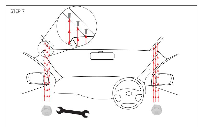
Using washers & Nyloc Nuts firmly tighten bolts in place.
