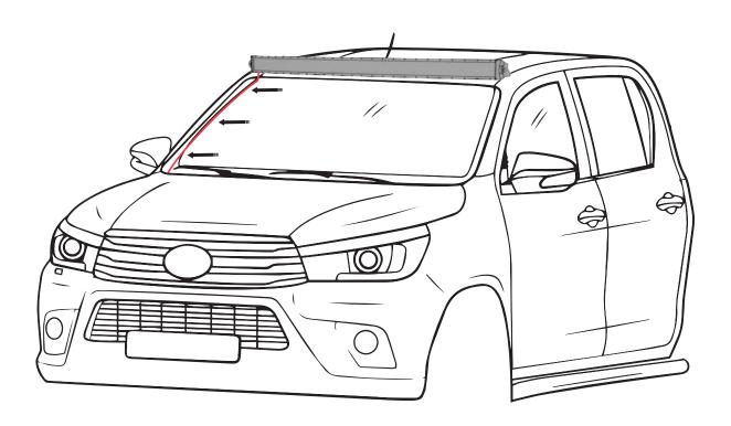
Run the wiring down the side of your windscreen, and reel under bonnet preferably on the same side as the battery. Use a few dabs of silicone or to hold it in place.
