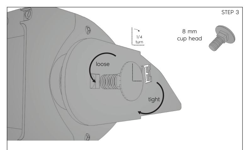
To adjust the Light bar, unwind the mount and turn bolt 1/4 clockwise or anti-clockwise in the square hole and refit it to the light bar.
