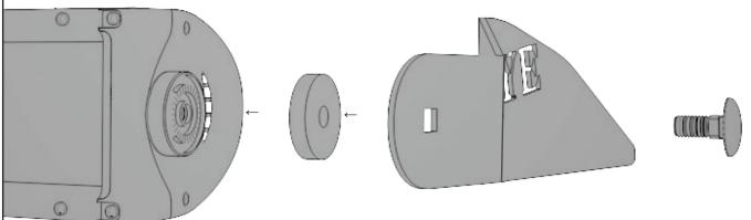
Wind the mounts onto the ends of the light bar, using the 8mm cup head bolts and rubber washers provided.
