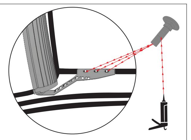
Silicone around the bolt threads, then place the Cup Head bolts into the drilled holes.
