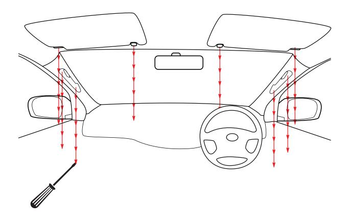
You will need to drop the roof lining on the driver's and passenger's corners.
