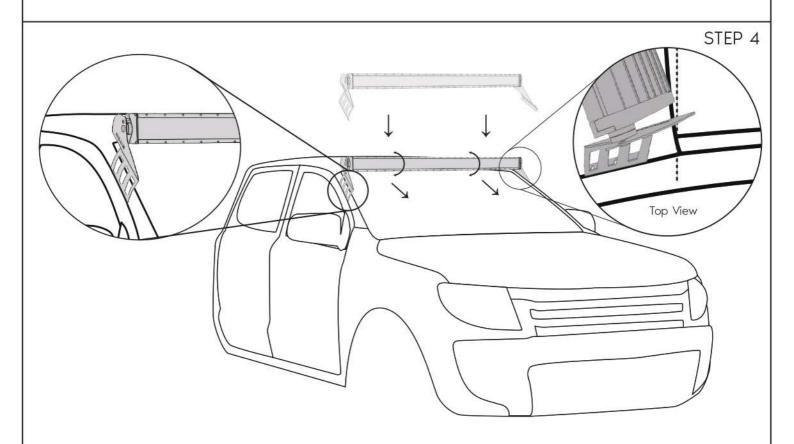
Place light bar into position on top of the windscreen, you will need a spare set of hands to help you hold it up there. The mounts sit on the A pillar in the Door jam. There is a limited area where these mounts can sit so they sit flush, and vertically on the vehicle. Adjust the light to sit horizontally.
