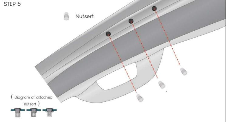
\*Tip: Ensure the drill bit is correct size.
