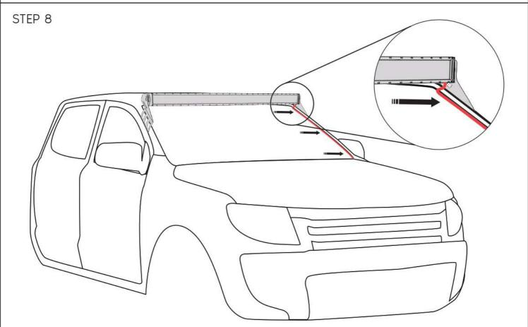
Run the wiring down the side of your windscreen, preferably on the same side as the battery. Use a few dabs of silicone or to hold it in place.
