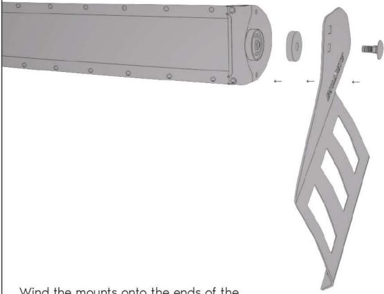
Wind the mounts onto the ends of the light bar, using the 8mm cup head bolts and rubber washers provided.
