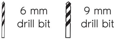
\*Tip: Pre-drill holes first with 6mm drill bit and then use 9mm.
