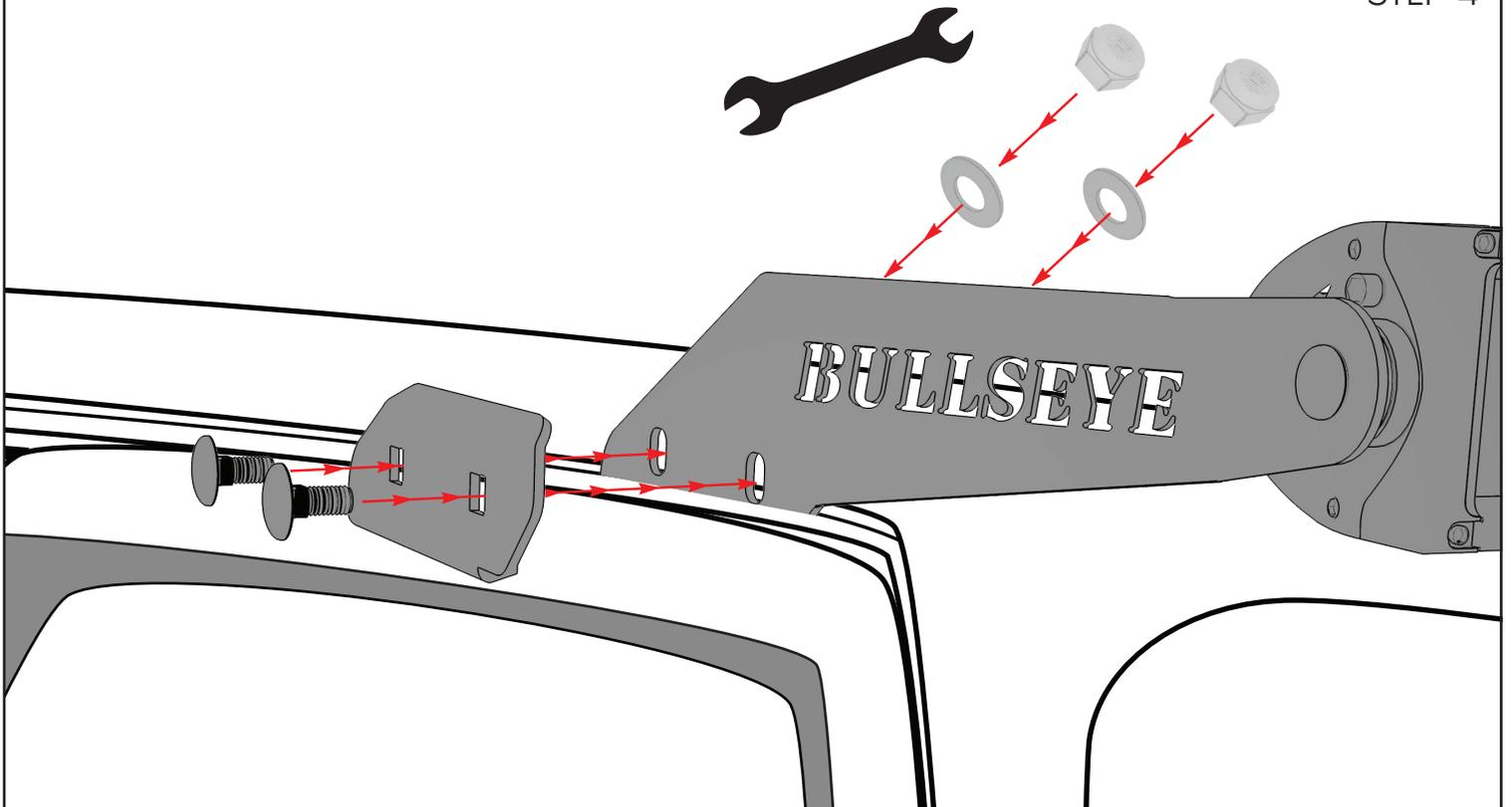
Hold the mount in place on the A Pillar in the gutter, using the 4 x 10mm cup head bolts and rubber washer provided, bolt the clamps onto the gutters and mounts.
