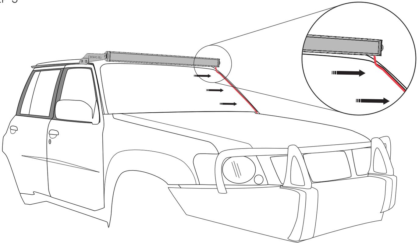
Run the wiring down the side of your windscreen, preferably on the same side as the battery. Use a few dabs of silicone or to hold it in place.
