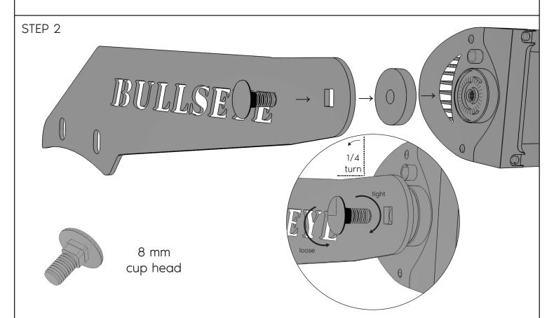
Wind the mounts onto the ends of the light bar, using the 8mm cup head bolts and rubber washers provided.
