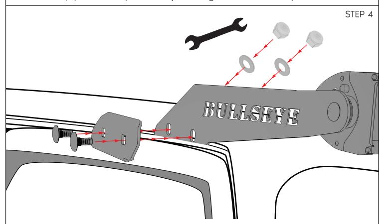
Hold the mount in place on the A Pillar in the gutter, using the  $4 \times 10$ mm cup head bolts and rubber washer provided, bolt the clamps onto the gutters and mounts.
