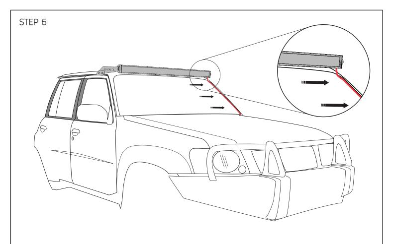
Run the wiring down the side of your windscreen, preferably on the same side as the battery. Use a few dabs of silicone or to hold it in place.
